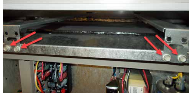
FIGURE 6 Remove Four Screws
