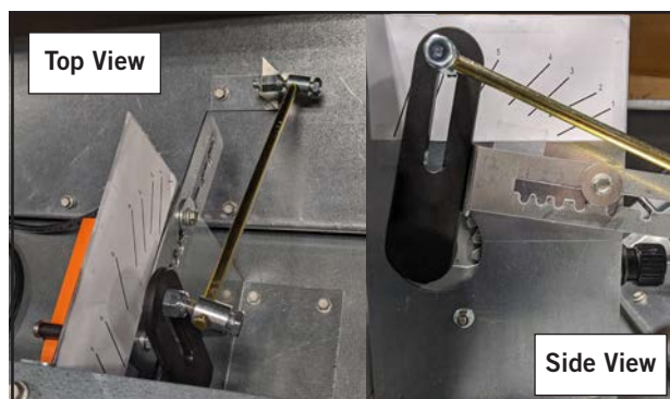
FIGURE 13 Take Blade Out of Shipping Position
