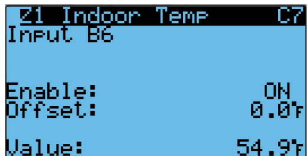
FIGURE 39 Enable/Disable Zone 1 Indoor Temperature Sensor
