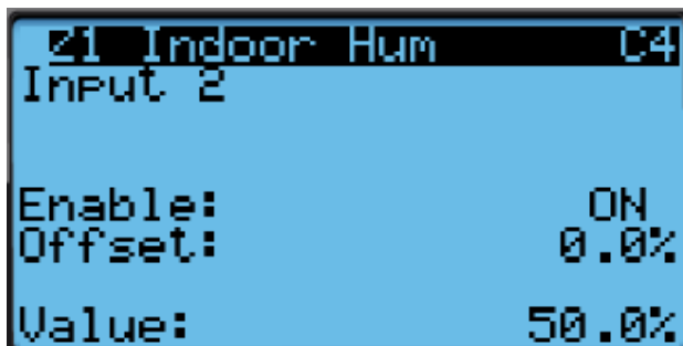
FIGURE 48 Adjusting Sensor Offset Value
