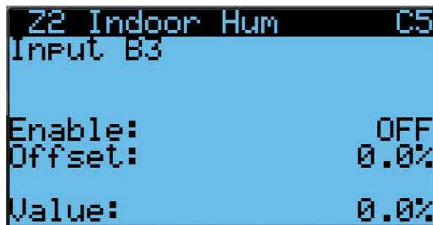
FIGURE 37 Enable/Disable Zone 2 Indoor Humidity Sensor
