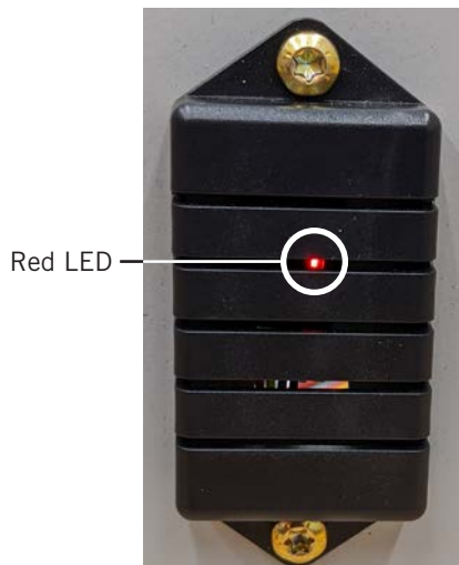
FIGURE 31 Verifying Sensor LED Is Illuminated
