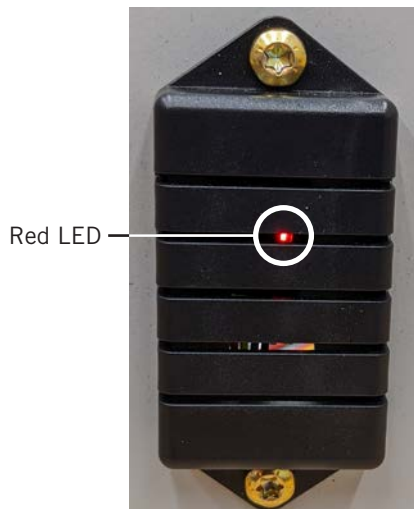
FIGURE 31 Verifying Sensor LED Is Illuminated
