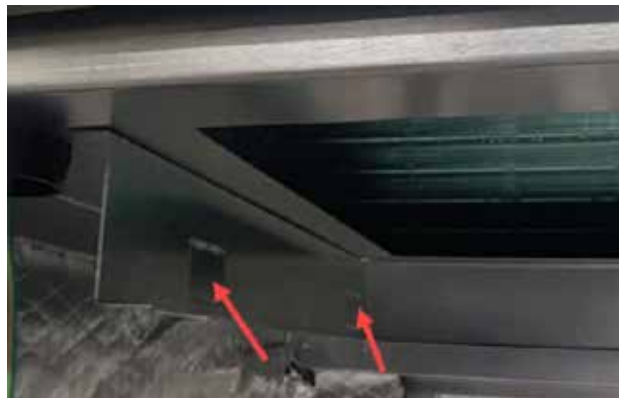
FIGURE 10 Bend Filter Tabs Down
