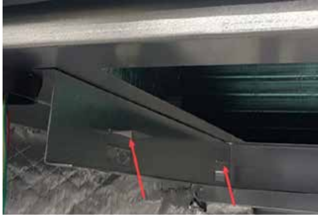
FIGURE 10 Bend Filter Tabs Down
