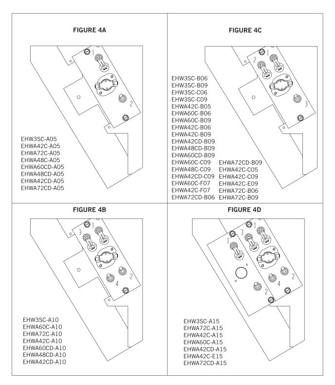
NOTE: THERMAL CUTOFFS TO BE AT TOP OF AIR FRAME WHEN INSTALLING.
