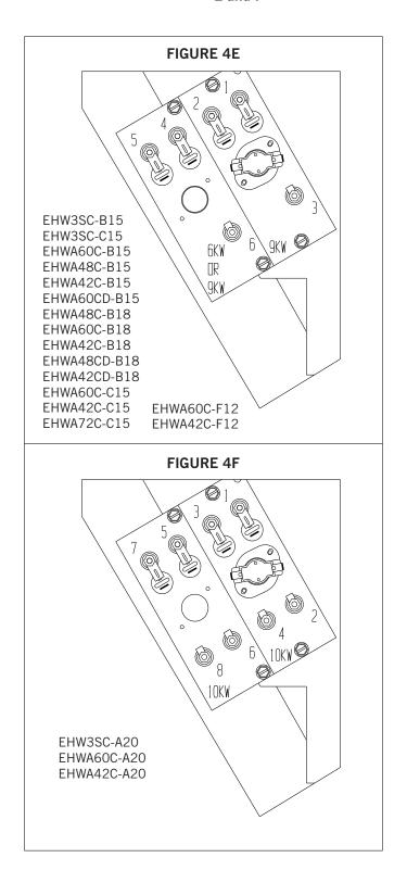
NOTE: THERMAL CUTOFFS TO BE AT TOP OF AIR FRAME WHEN INSTALLING.
