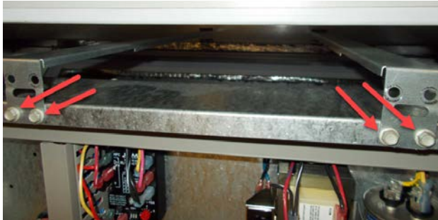
FIGURE 38 Remove Four Screws
