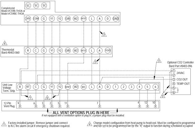
Do not connect "A" from thermostat if optional CO2 controller is used 0-10 VDC modulating C02 control signal for modulating ventilation control (optional for ECON only - see vent instruction manuals) 3
