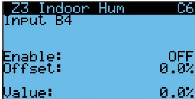
FIGURE 38 Enable/Disable Zone 3 Indoor Humidity Sensor
