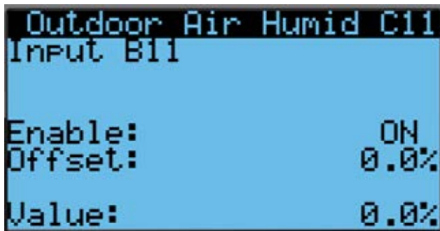
FIGURE 43 Enable/Disable Outdoor Air Humidity Sensor
