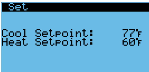
FIGURE 19 Cool and Heat Setpoints
