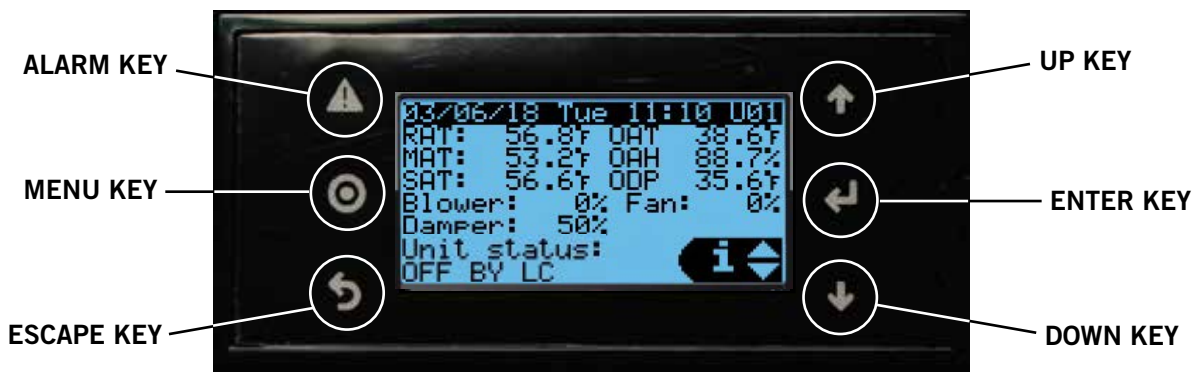
FIGURE 36 TEC-EYE (Bard P/N 8301-059) Display and Interface (Status Screen Shown)
