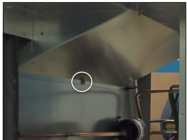
FIGURE 7 Remove Screw from Condenser Partition Insert
