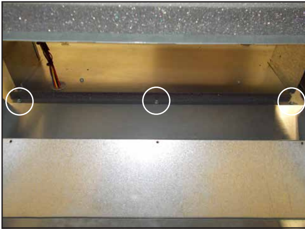
FIGURE 8 Remove Screws from Condenser Partition Insert
