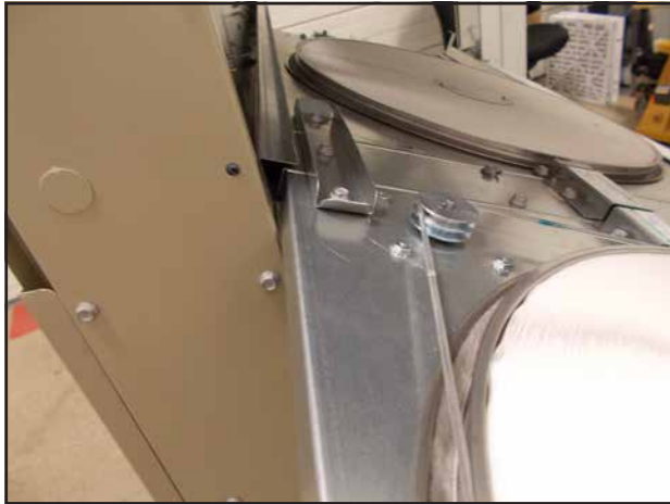
FIGURE 30 Slide Cassette Frame into Mounting Rails
