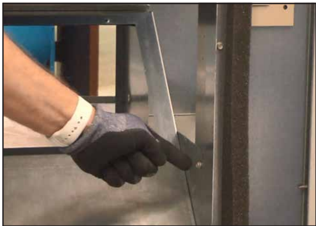
FIGURE 9 Remove Screws from Sides of Condenser Partition Insert
