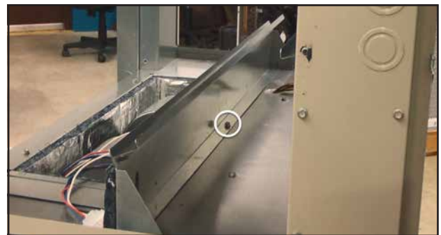
FIGURE 16 Install Center Cassette Rack
