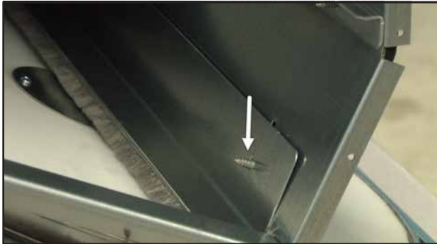
FIGURE 42 Loosen Screws to Adjust Pile Seal
