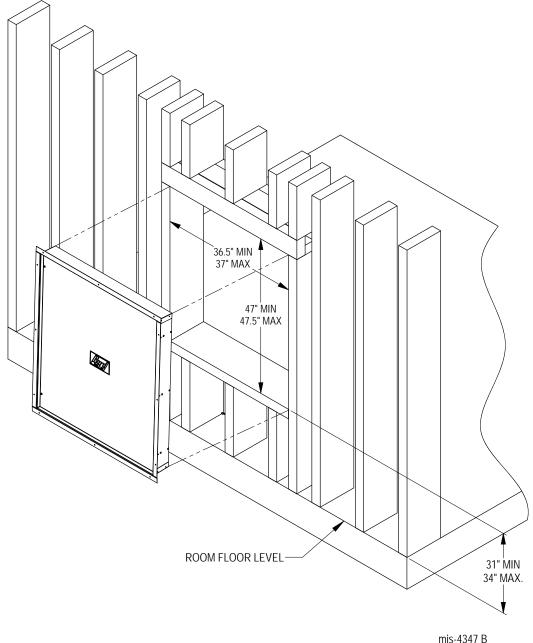
secured to the wall by using two (2) field-supplied wood screws through the holes in the bottom mounting flange of the sleeve. The sleeve must be checked to make sure that it is square in the opening. Once the sleeve is square, the side and top mounting flanges of the sleeve must be secured to the wall with ten (10) field-supplied wood screws through the holes in the flanges.
