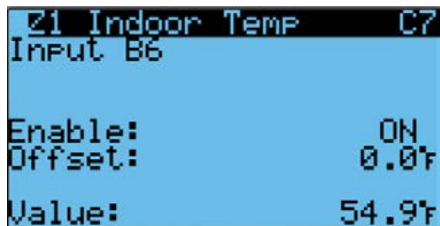
FIGURE 37 Enable/Disable Zone 1 Indoor Temperature Sensor
