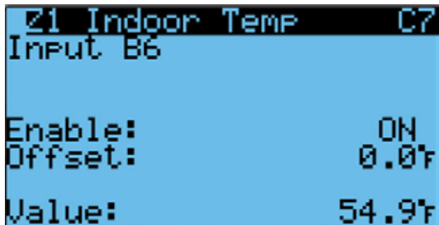
FIGURE 37 Enable/Disable Zone 1 Indoor Temperature Sensor
