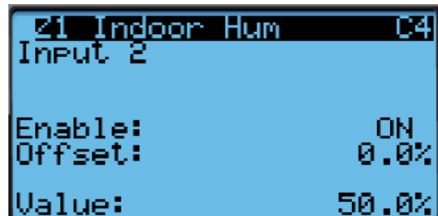
FIGURE 46 Adjusting Sensor Offset Value
