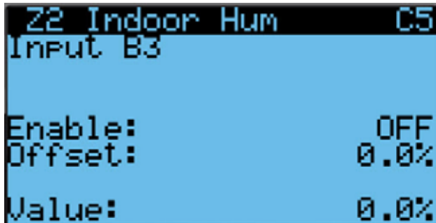
FIGURE 35 Enable/Disable Zone 2 Indoor Humidity Sensor
