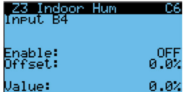
FIGURE 46 Enable/Disable Zone 3 Indoor Humidity Sensor
