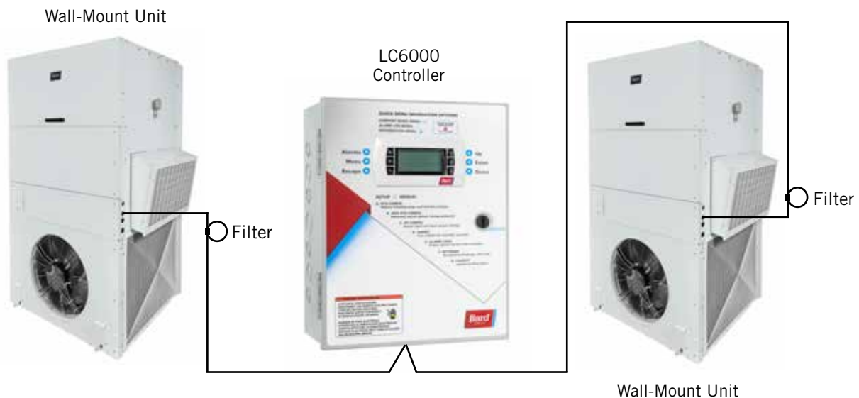
FIGURE 21 Communication Wiring (Alternate Method)
