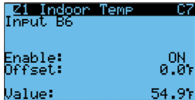
FIGURE 39 Enable/Disable Zone 1 Indoor Temperature Sensor
