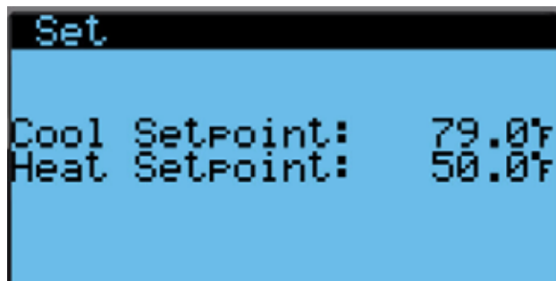
FIGURE 18 Cool and Heat Setpoints
