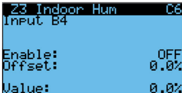
FIGURE 36 Enable/Disable Zone 3 Indoor Humidity Sensor
