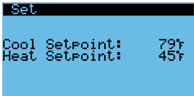
FIGURE 19 Cool and Heat Setpoints
