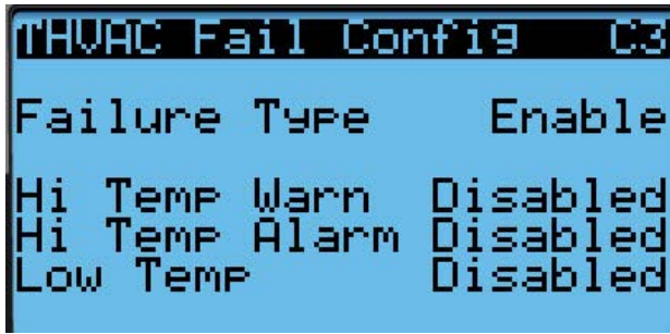
FIGURE 46 Changing HVAC Fail Outputs
