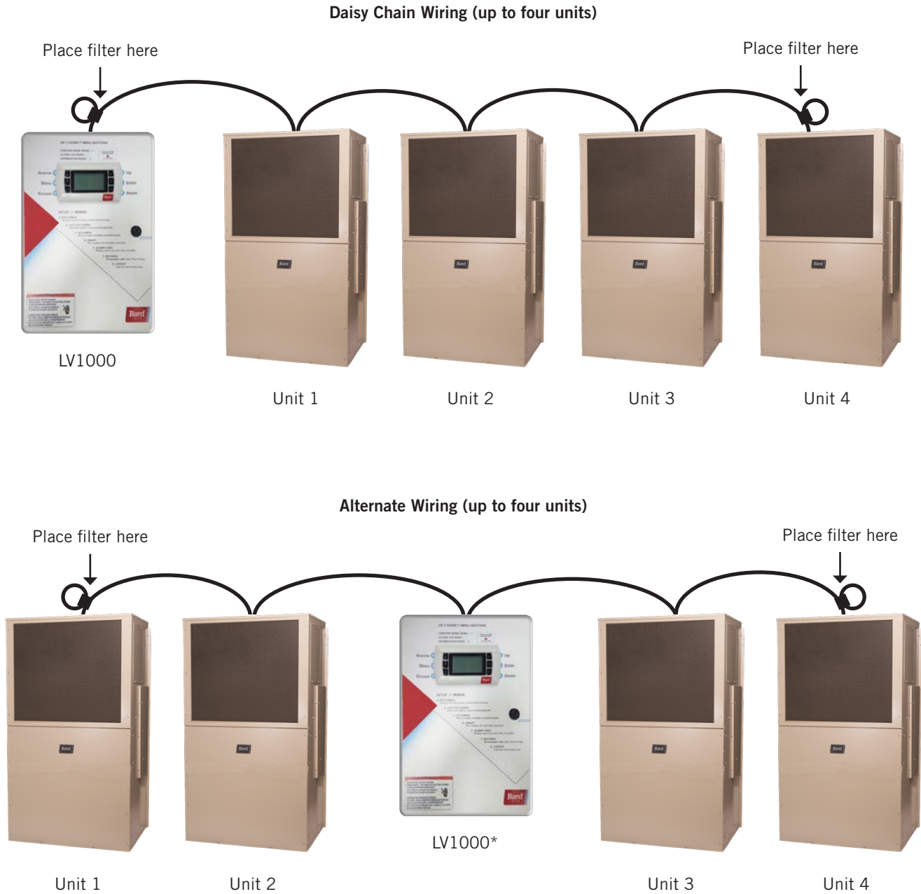
FIGURE 11 Placement of Communication Wire Filters (Daisy Chain and Alternate Methods)
