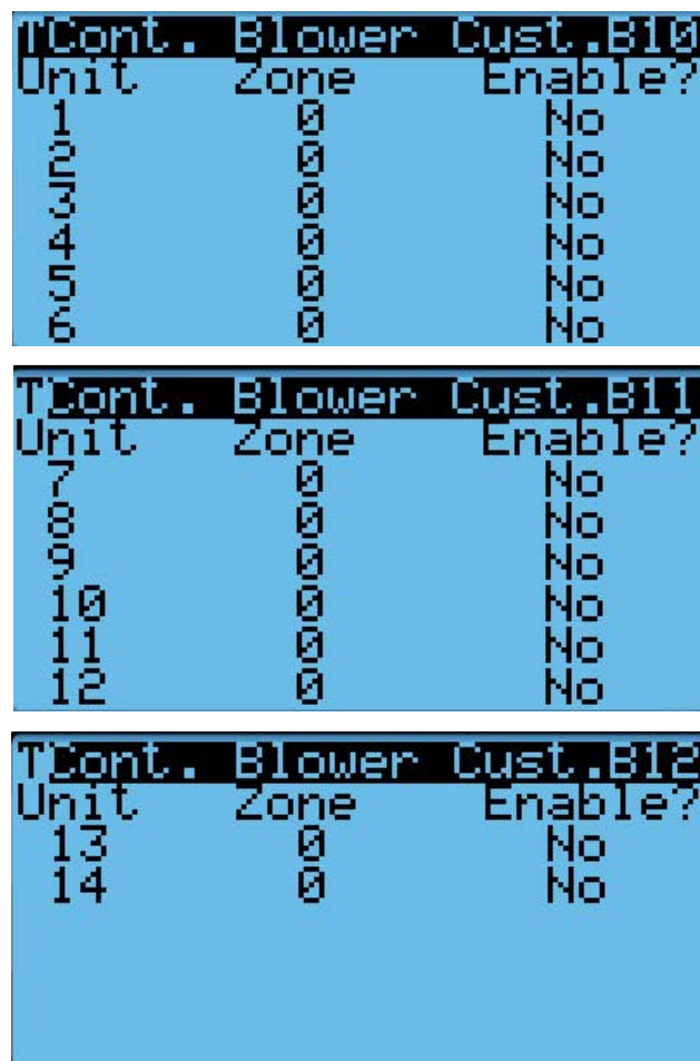
FIGURE 35 Continuous Blower Custom Configuration
