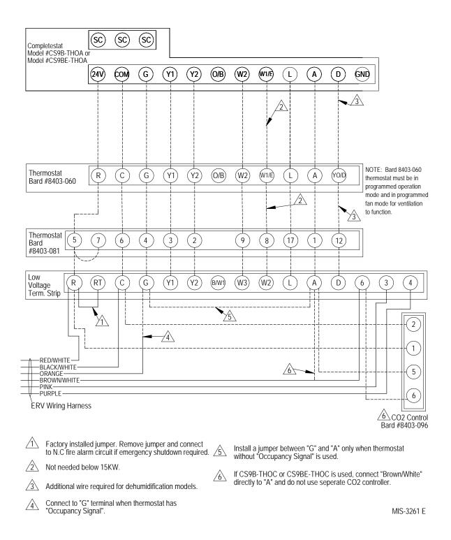
FIGURE 18 Air Conditioner with ERV and CO<sub>2</sub> Control (Fully Modulating) ("R" Vent Code)
