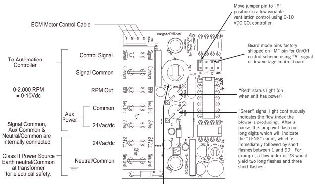
**CONFIGURING BARD PART #8403-096 CO<sub>2</sub> CONTROL for CRV MODULATING CONTROL**
