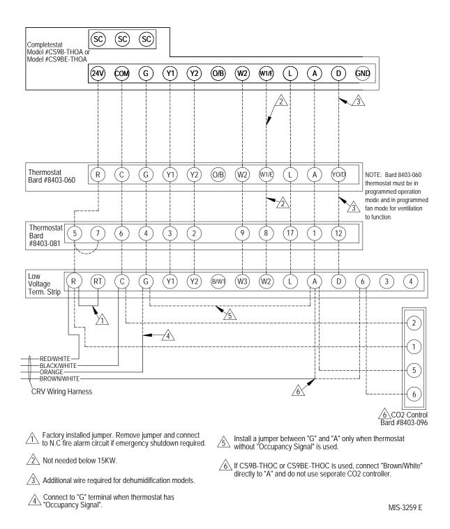
FIGURE 16 Air Conditioner with ERV, without  $CO_2$  Control ("R" Vent Code)
