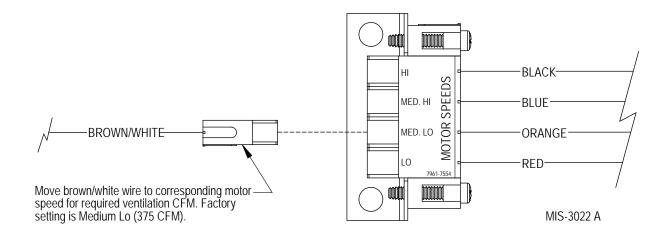
FIGURE 22 CRV Speed Change Terminal Access
