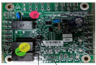
O/V Jumper TEST Jumper
