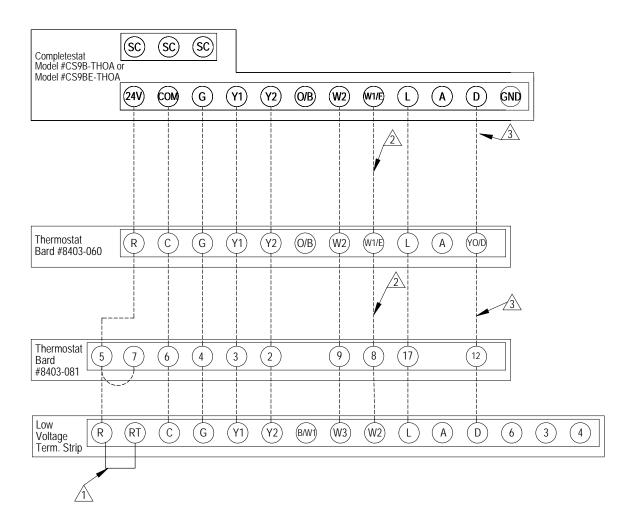
A Factory installed jumper. Remove jumper and connect to N.C fire alarm
