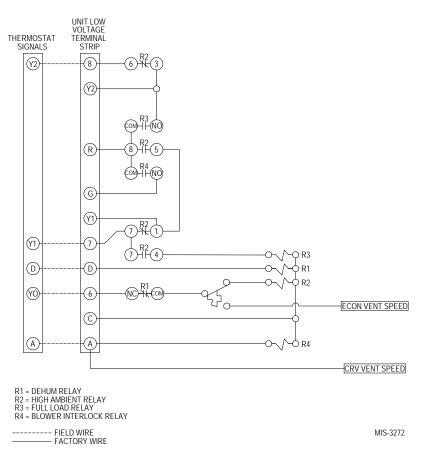
FIGURE 23 Economizer Control Circuit
