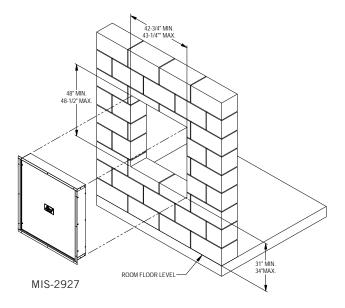
inside to the outside. This will allow any water that gets into the sleeve to drain out. Once the test fitting has been checked out, the sleeve should be removed from the wall.
