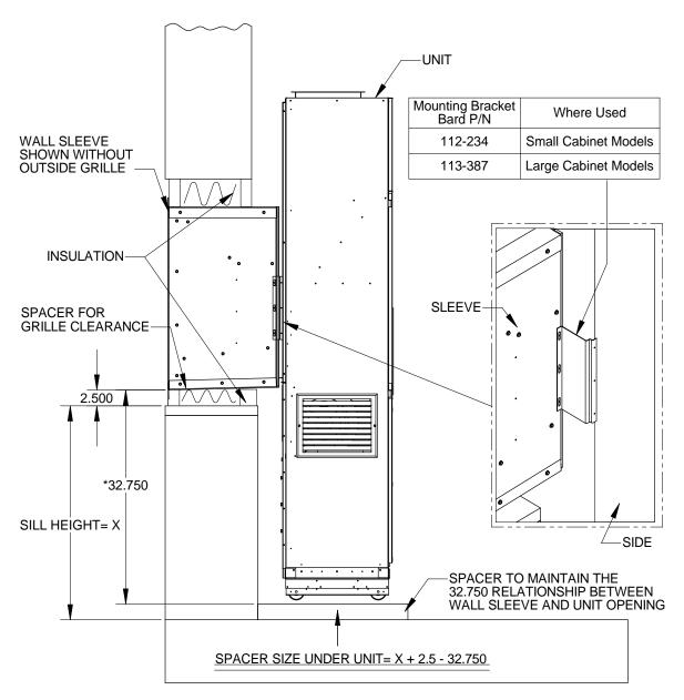
\*THIS DIMENSION MUST REMAIN CONSTANT WHEN FABRICATING UNIT AND WALL SLEEVE REGARDLESS OF THE WINDOW SILL DIMENSIONS
