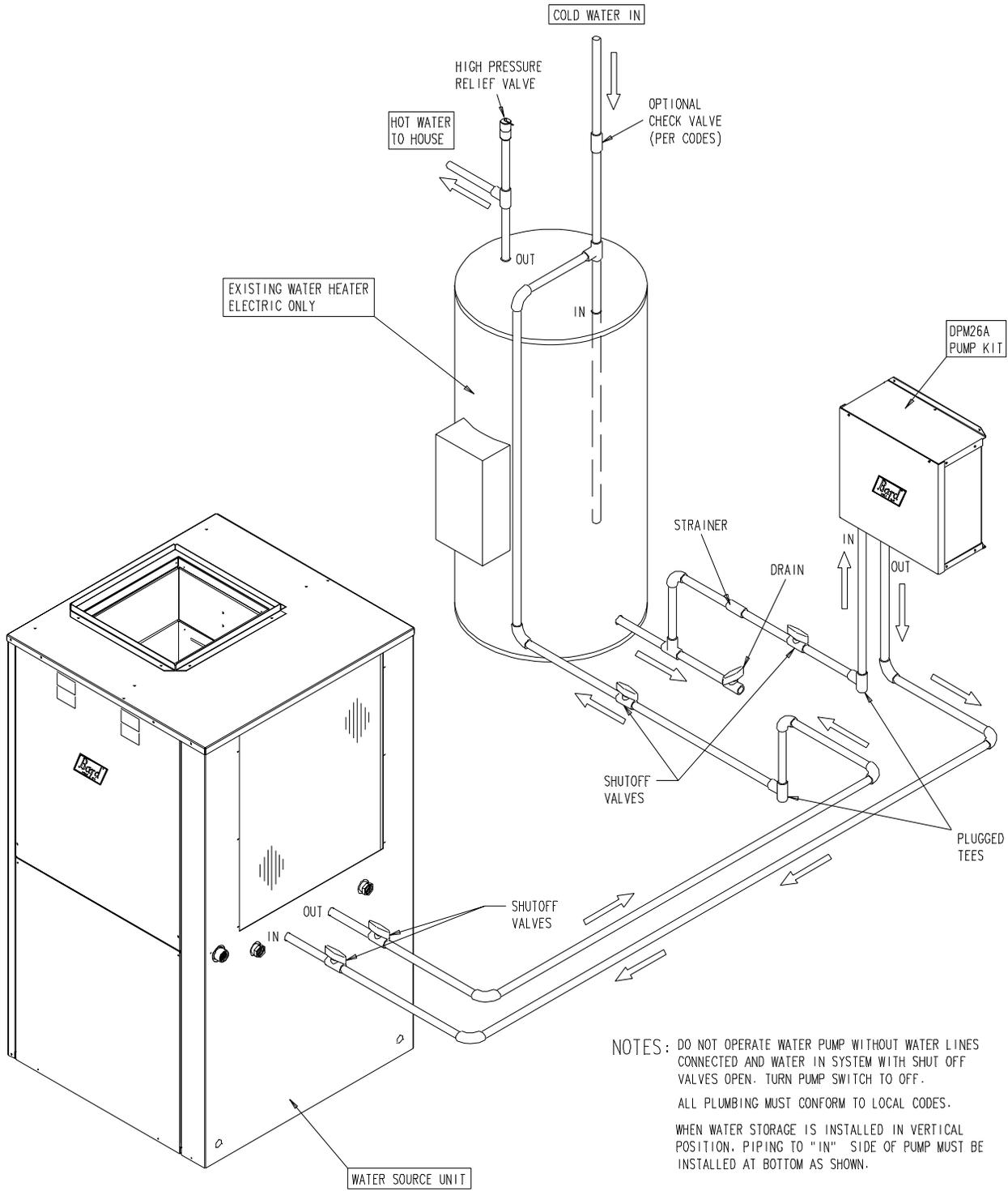
NOTES: DO NOT OPERATE WATER PUMP WITHOUT WATER LINES CONNECTED AND WATER IN SYSTEM WITH SHUT OFF VALVES OPEN. TURN PUMP SWITCH TO OFF.
