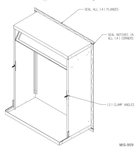
Once the opening is framed, the sheeting can be installed; the sheeting material must not extend into the opening.
