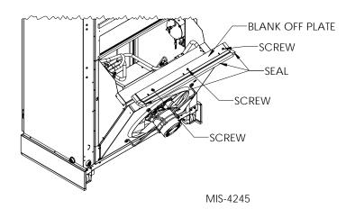
Bypassing the outdoor drain pan with the indoor condensate can benefit the installation in regards to reducing growth within the lower pan by prohibiting standing water during the warm cooling season.
