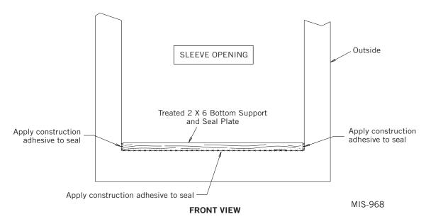
FIGURE 3 **Application of Sealant to Flanges**
