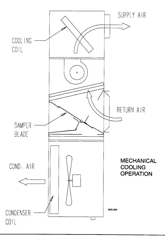
Figure 7 - Damper Position - Full Closed
