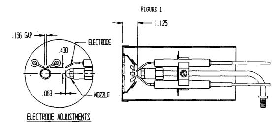
Gun Assembly Adjustment. The qun assembly can be adjusted in the slot inside of fan housing by loosening screw holding slot cover in position. Nozzle tip should ordinarily be located 1-1/8" behind the front face of the cone.
