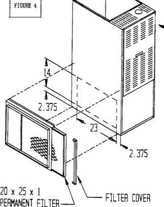
To remove filter from the filter rack, remove the filter access cover and grasp the end of the filter. This filter is the permanent high velocity type foam filter which may be washed and used over and over. DO NOT replace it with a fiberglass disposable filter of the same size.
