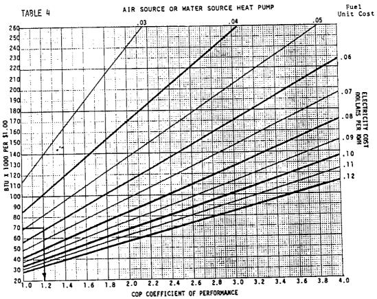
Determine Economic Balance Point for Heat Pump when used with an oil furnace of 65% AFUE 6 \$1.30 per gallon for oil from example 1 (oil furnace 70,000 Btuh/%) and electric rate of .06 kWh. A 1.21 COP, heat pump and oil is equal in operating cost. Example 2.
