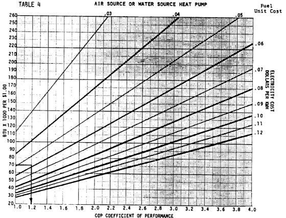
Example 2. Determine Economic Balance Point for Heat Pump when used with an oil furnace of 65% AFUE 6 \$1.30 per gallon for oil from example 1 (oil furnace 70,000 Btuh/%) and electric rate of .06 kWh. A 1.21 COP, heat pump and oil is equal in operating cost.
