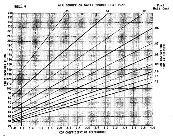
Example 2. Determine Economic Balance Point for Heat Pump when used with an oil furnace of 65% AFUE 6 \$1.30 per gailon for oil from example 1 (oil furnace 70,000 Btuh/\$) and electric rate of .06 kWh. A 1.21 COP, heat pump and oil is equal in operating cost.
