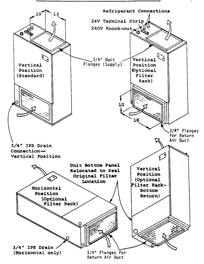
NOTE: If no return air duct is used, applicable installation codes may limit this cabinet to installation only in a single story structure.
