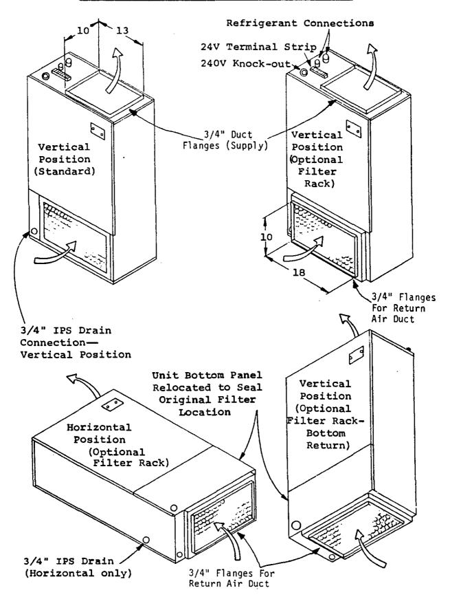
NOTE: If no return air duct is used, applicable installation codes may limit this cabinet to installation only in a single story structure.
