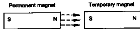
Hard alloy steel Permanent magnet Soft iron Temporary magnet Magnetic induction—permanent magnet induces a magnetic field in soft iron bar with opposite polarity shown. Temporary magnet loses its magnetic field when separated from permanent magnet.
