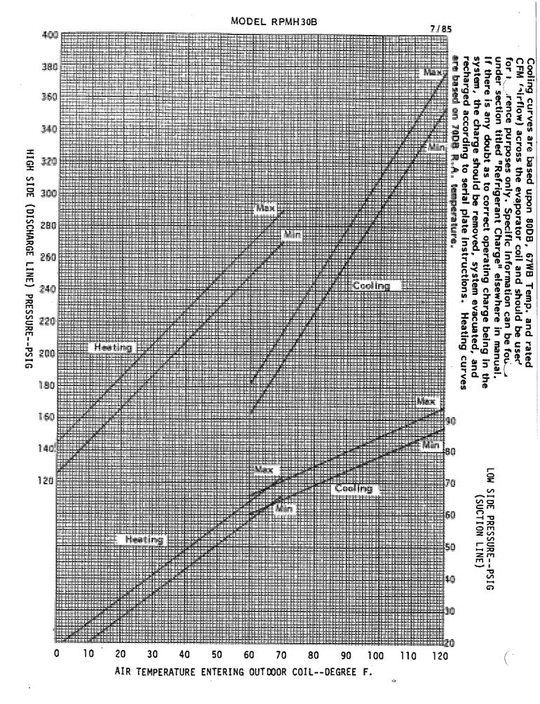
Cooling curves are based upon 80DB, 67WB Temp. and rated
