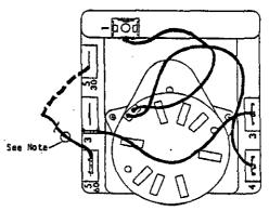
NOTE: All models are connected to 5/60 terminal (60 minute).
