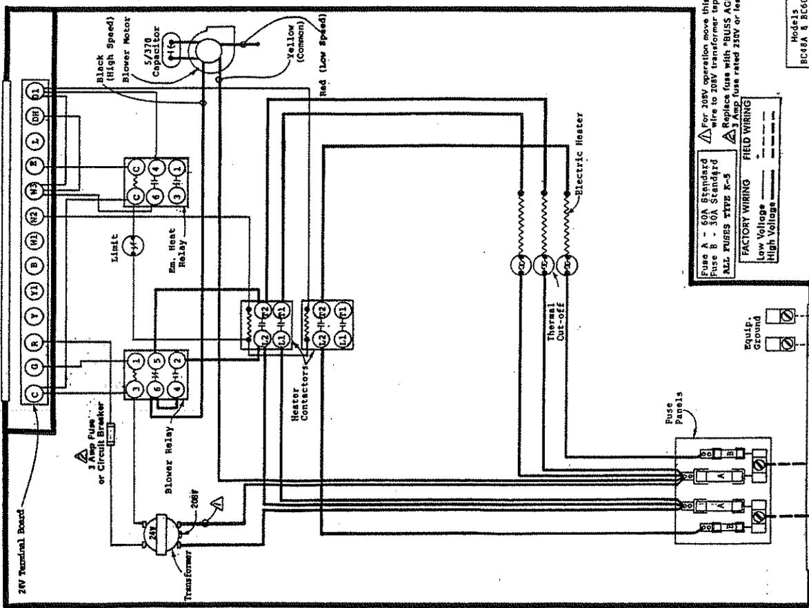
For 208V operation move this wire to 208V transformer tap.
