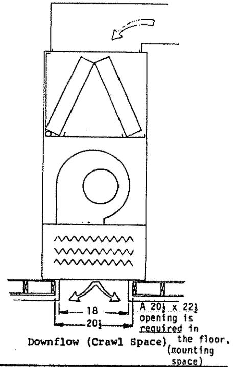
**WARNING:** Failure to provide the one inch clearance for the first two feet between the supply duct and a combustible surface can result in fire.
