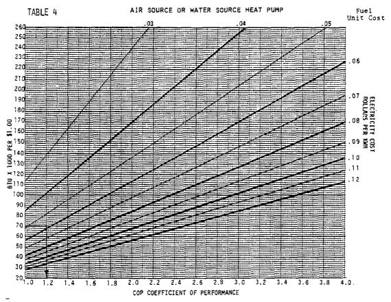
Example 2. Determine Economic Balance Point for Heat Pump when used with an oil furnace of 65% AFUE % \$1.30 per gallon for oil from example 1 (oil furnace 70,000 Btuh/%) and electric rate of .06 kWh. A 1.21 COP, heat pump and oil is equal in operating cost.
