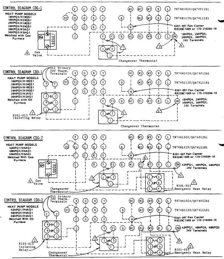
Outdoor thermostat range 0 to 70°F. Normally set at 40-45°F. Changes operation from heat pump to fossil fuel furnace as outdoor temperature falls below setpoint. Cut-in approximately 5°F differential (switches on temperature rise approximately 5°F above setpoint). Locate in outdoor unit control box. See section "Gas or Oil Furnace Applications" before any other setting is used. Remove jumper Y-Y1.
