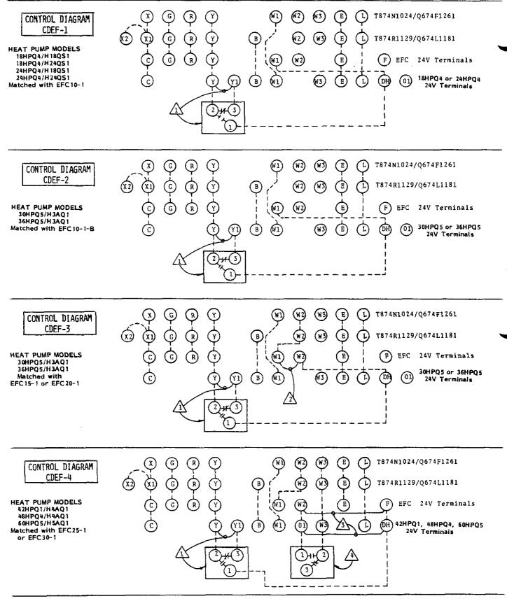
If optional compressor cut-off, ODT-070 is used, remove jumper Y-Y1.
