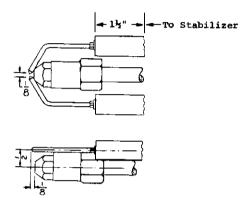
Gun Assembly Adjustment. The gun assembly can be adjusted in the slot inside of fan housing by loosening screw holding slot cover in position. Nozzle tip should ordinarily be located 5/16 inch behind the front face of the cone.
