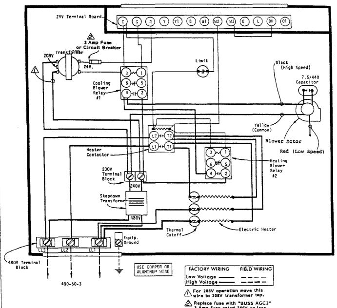
Replace fuse with "BUSS AGC3" 3 Amp fuse rated 250V or less.
