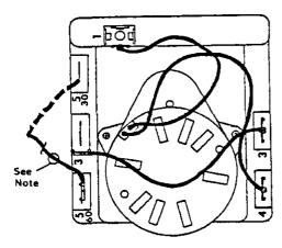
NOTE: All models are connected to 5/60 terminal (60 minute).
