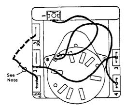
NOTE: All models are connected to 5/60 terminal (60 minute). Any model can be changed from 60 minutes to 30 minutes by unplugging from 5/60 terminal and reconnecting to 5/30 terminal as shown by dotted line.
