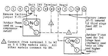
WALL THERMOSTAT AND SUBBASE COMBINATIONS
