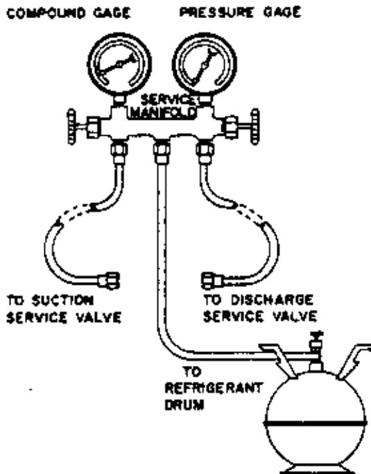
**ATTACHING GAUGE MANIFOLD**
