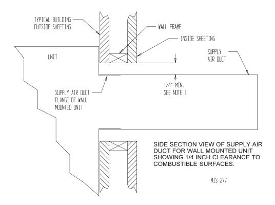
NOTE: A 1/4 inch clearance to combustible material for the first 3 feet of duct attached to the outlet air frame is required. However, it is highly recommended that a 1-inch clearance is used for ease of installation and maintaining the required clearance to combustible material
