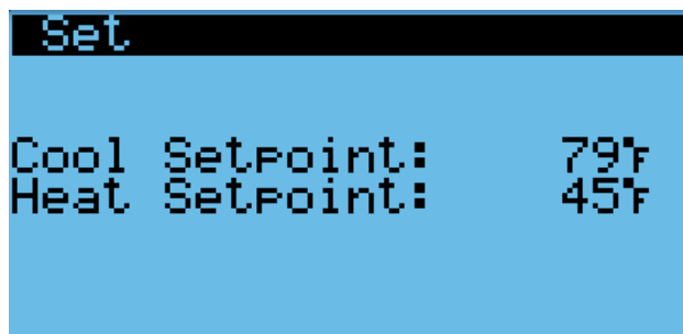
FIGURE 4 Cool and Heat Setpoints
