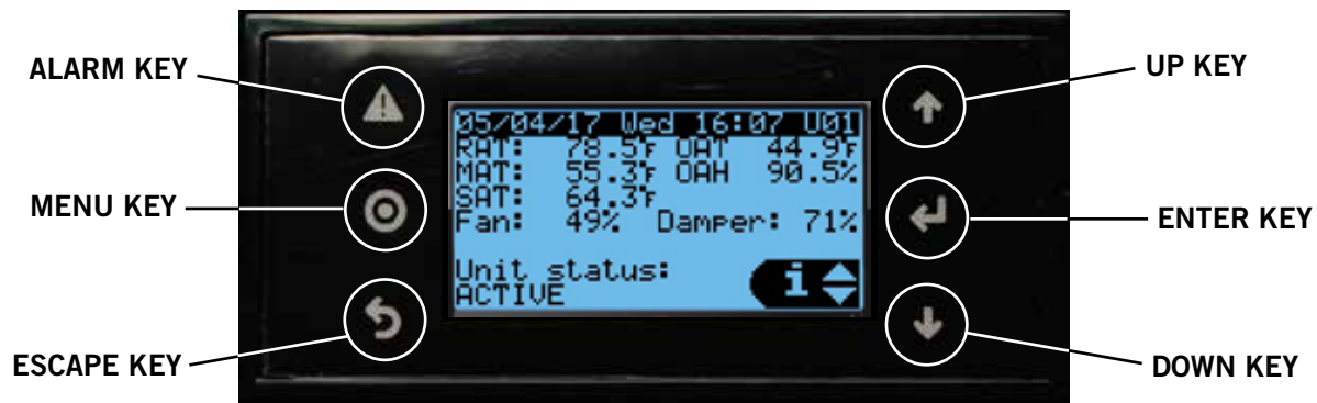
FIGURE 32 TEC-EYE™ (Bard P/N 8301-059) Display and Interface (Status Screen Shown)
