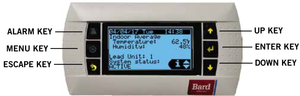
FIGURE 37 LV1000 Controller Display and Interface (Status Screen Shown)
