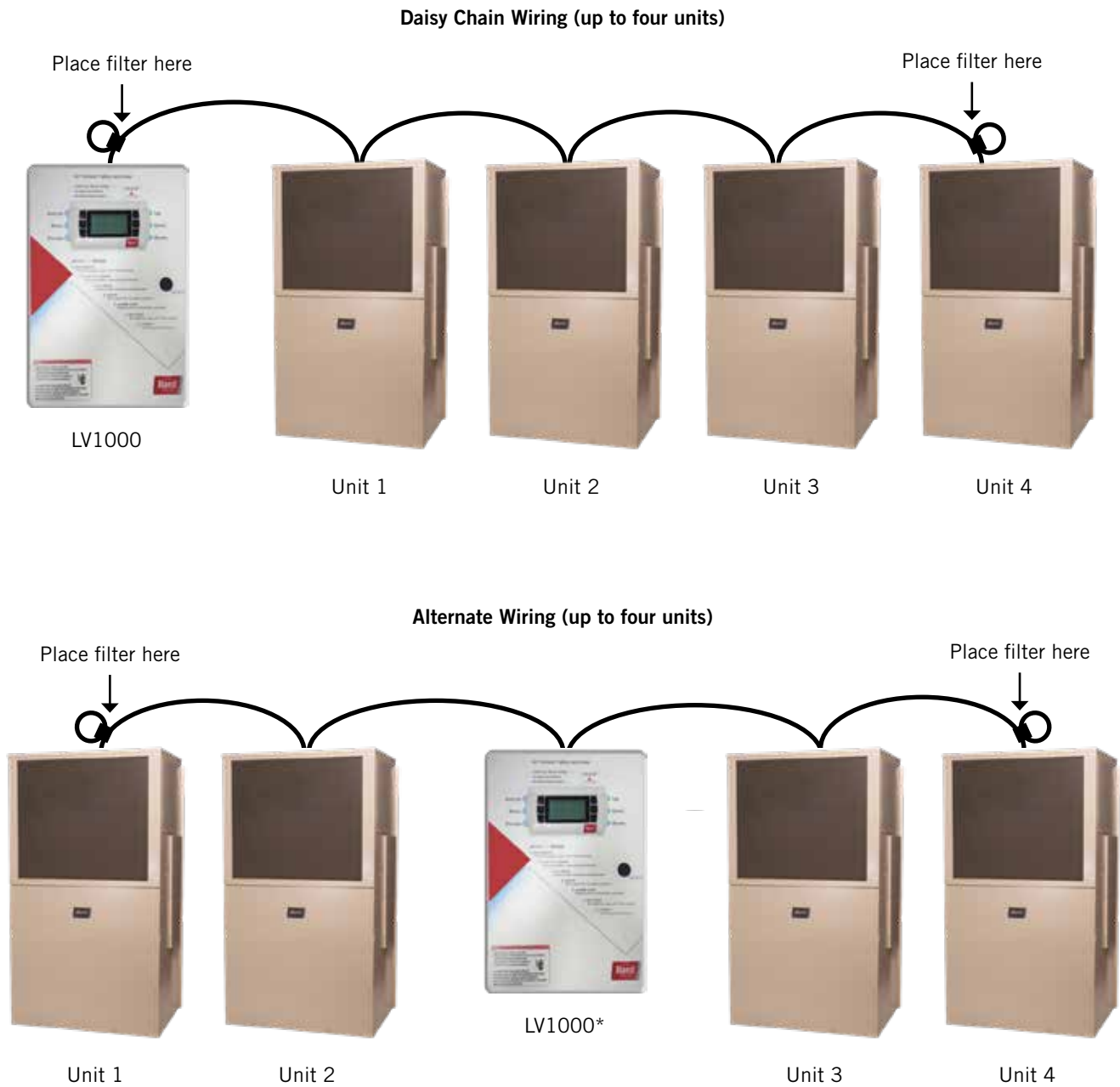
FIGURE 25 Placement of Communication Wire Filters (Daisy Chain and Alternate Methods)
