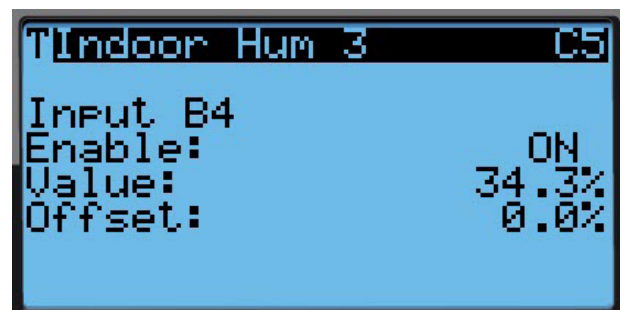
FIGURE 41 Configuring Indoor Humidity 3 Sensor
