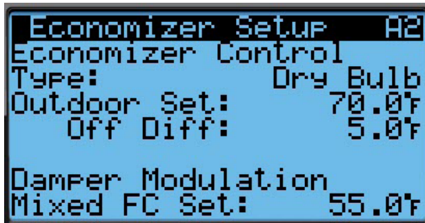
FIGURE 33 Changing Economizer Control Type
