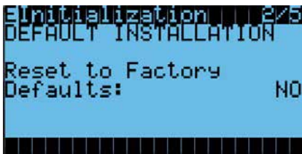
FIGURE 49 Restoring Factory Default Settings
