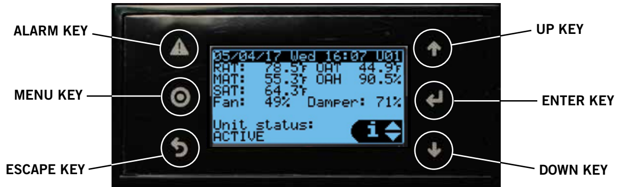
FIGURE 31 TEC-EYE™ (Bard P/N 8301-059) Display and Interface (Status Screen Shown)
